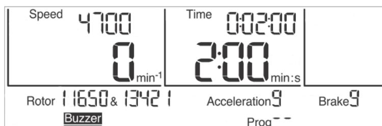
Fig. 20: The sound signal "Buzzer" is activated
