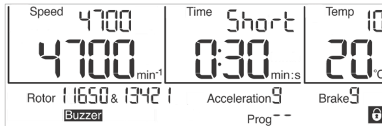
Fig. 16: Indication "Short" during a short run
