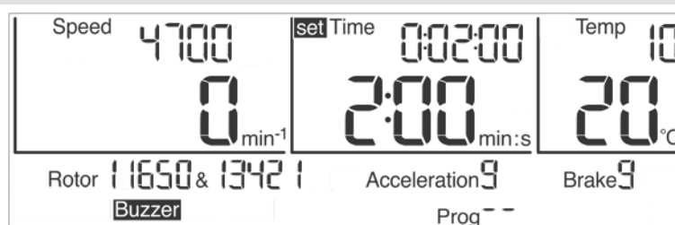
Fig. 13: Setting the runtime, here in the time unit "min:s"
