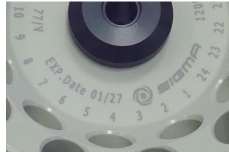
Fig. 4: Different service life – engraving on the bucket/rotor
