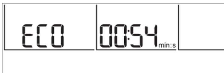
Fig. 29: Indication of the last 29 minutes of the countdown before the activation of the Eco mode
