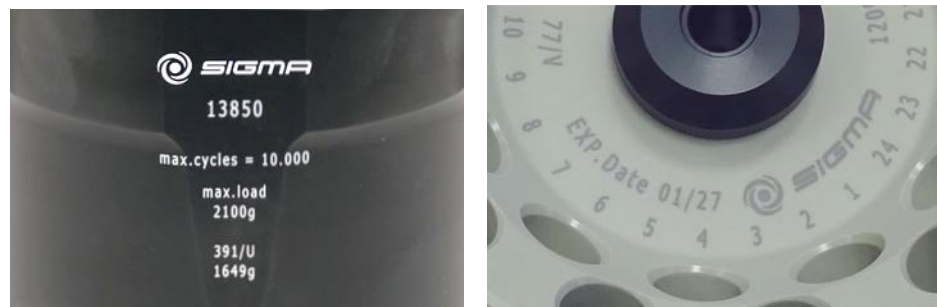
Fig. 5: Different service life – engraving on the bucket/rotor
