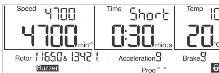
Fig. 18: Indication "Short" during a short run
