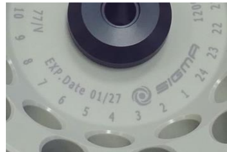
Fig. 4: Different service life – engraving on the bucket/rotor
