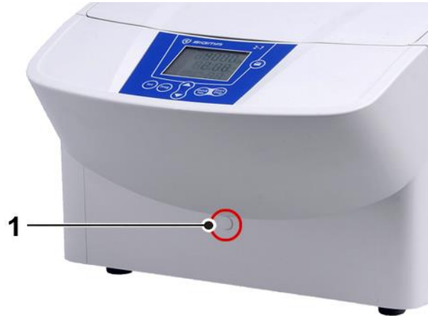
Fig. 10: Position of the opening for the emergency lid release
