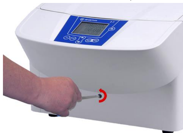
Fig. 11: Manual release of the lid lock
