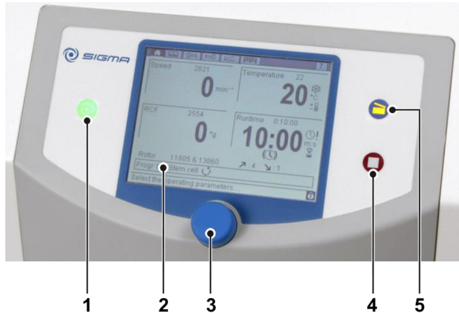
Fig. 10: User interface of the Spincontrol S control system
