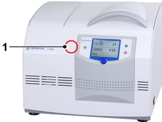
Fig. 30: Position of the opening for the emergency lid release
