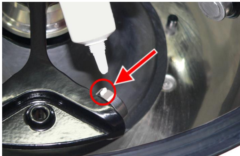
Fig. 32: Sufficient quantity of grease for one bolt
