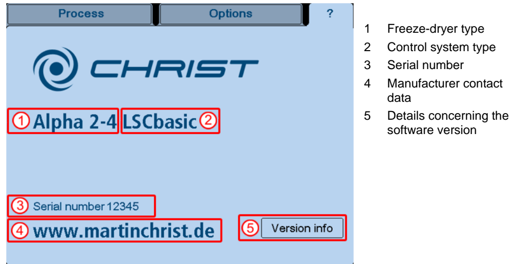
Fig. 48: Freeze-dryer system information (example)
