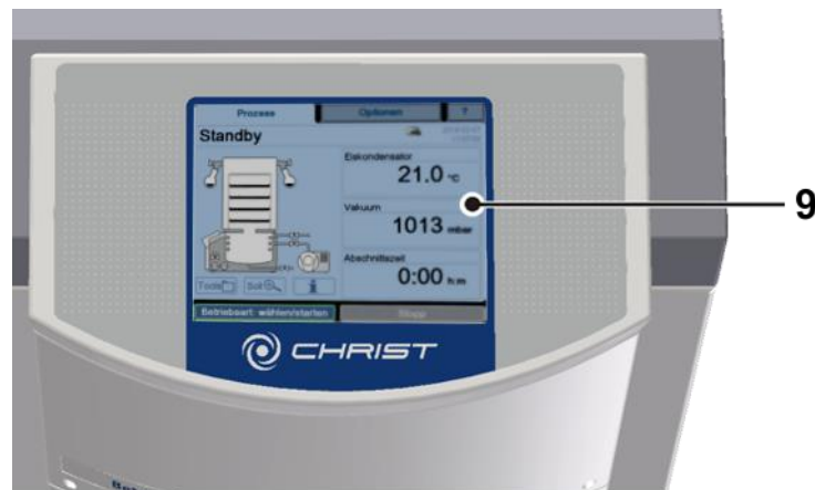
Fig. 4: User interface with touchpanel
