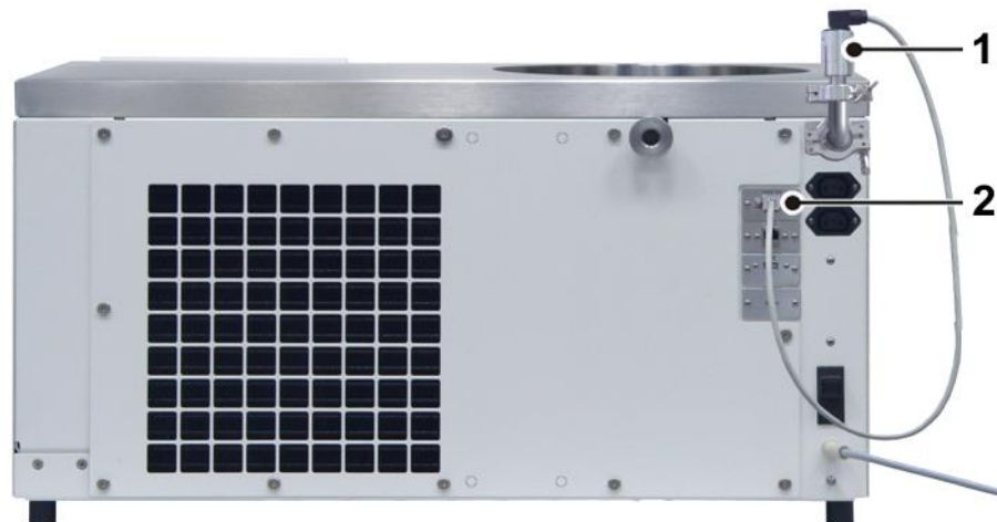
Fig. 11: Position of the vacuum sensor and the connection socket
