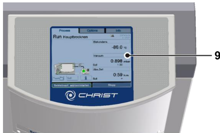
Fig. 60: User interface with touchpanel
