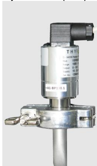
Fig. 12: Vacuum sensors of different manufacturers
