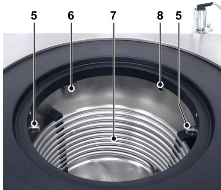
Fig. 73: Ice condenser chamber
