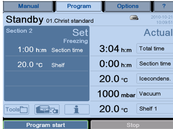
Fig. 64: The freeze-drying process can be started with the aid of the button "Program start".
