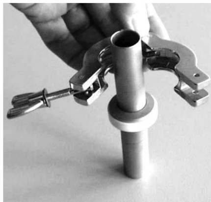
Fig. 67: Attaching the clamping ring
