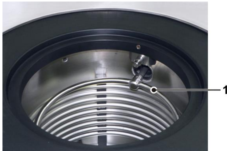
Fig. 10: Ice condenser chamber with a hot-water defrosting system
