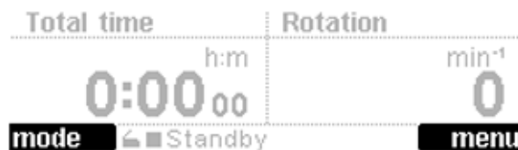
Fig. 20: Display of the assignment of the function keys; here: left key "mode", right key "menu"
